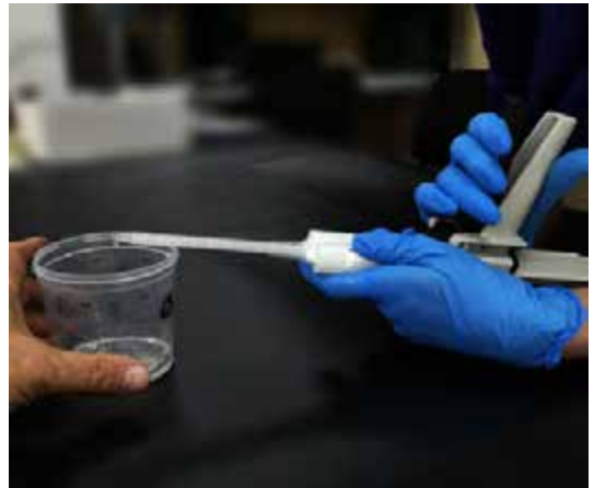
16. Purge small amount of resin from mixer to remove air. Incline gun and mixer to assist airflow.
