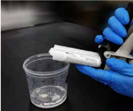
13. Purge cylinders until resin exits from both openings, inclining gun lower than receptacle.
